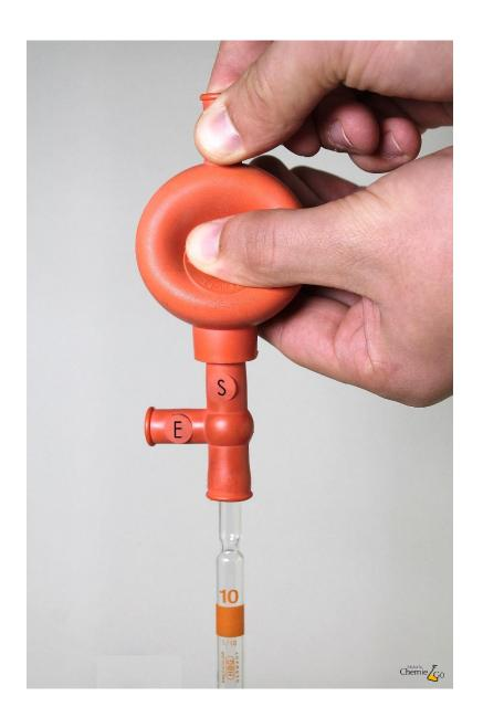
Valve **A** is opened by squeezing. Air can be released from the pipette filler by simultaneously squeezing valve A and the bulb.
