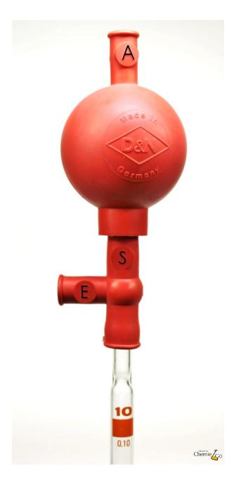
The top of the pipette is inserted in the bottom of the rubber bulb as shown in on the left.
