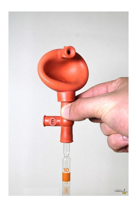
In order to take up liquid into the pipette, valve **S** is opened by squeezing.
